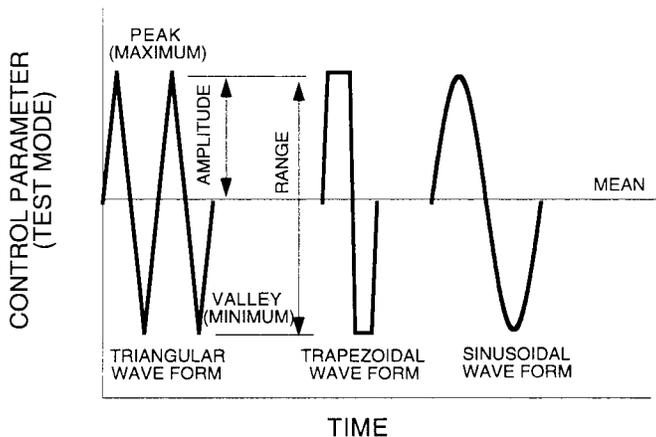
**FIG. 1 Cyclic Fatigue Nomenclature and Wave Forms**
